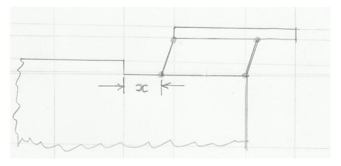
The critical value here is x, the length of the rods. This is given by:
