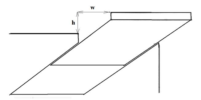
Conceptually simpler, indeed, but more complex in operation: the platform must be maintained in its raised position actively, by the hydraulics, or by some additional locking mechanism. The previous arrangement is purely mechanical in operation, and can be maintained in its raised position statically, by struts beneath the plank.
