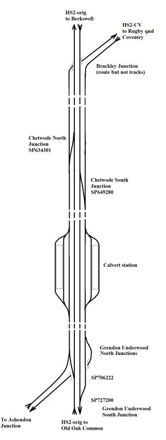
The article Same Speed Railways, Appendix B, gives extensive information on HS Junctions, layout of stations, acceleration and deceleration distances and times. The following track diagrams, while purely topological, follow the above conventions exactly.
